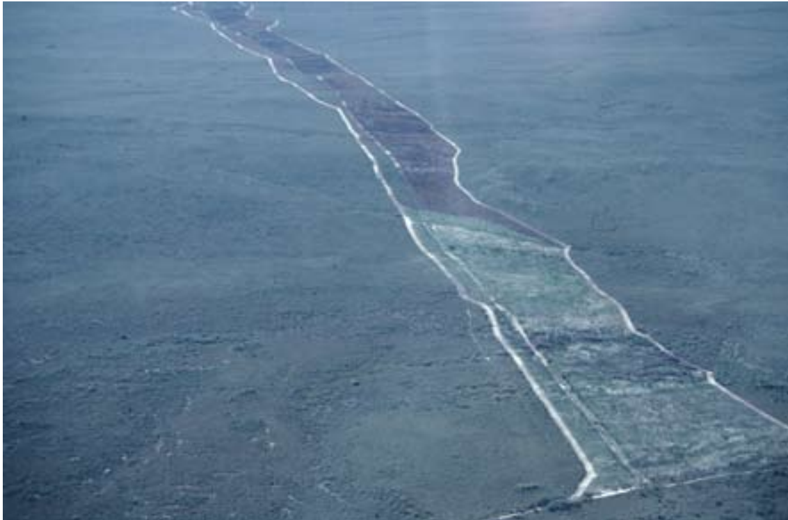
Plate 2.1 Road and track networks: parallel tracks placed to enable between-track burning for the creation of a buffer strip on the coastal plain north of Perth, Western Australia (Gill 1985).
